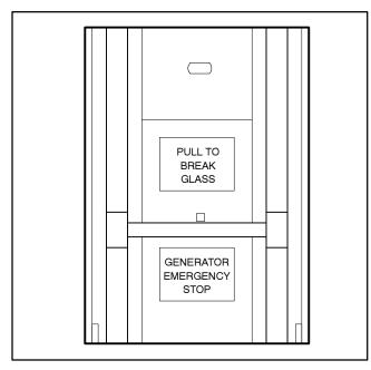
Figure 7-8 Remote Emergency Stop Switch
